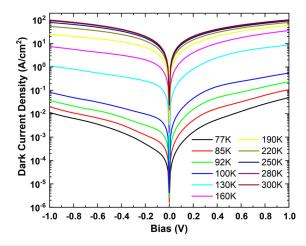
**FIG. 4.** Dark current density-bias voltage curves of the SML QD-QCD with a diameter of 130  $\mu$ m measured from 77 to 300 K.
