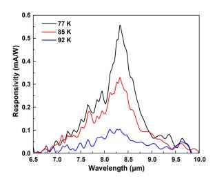
**FIG. 6.** Photoresponse under the normal incidence of the SML QD-QCD device measured at 77 K,  $85\,\rm K$ , and  $92\,\rm K$  under zero bias.
