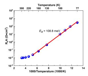
**FIG. 5.**  $R_0A$  product-inverse temperature dependences of the 130  $\mu$ m diameter device. The blue dots are  $R_0A$  values from 77 K to 300 K, and the red line is the fitted curve with the Arrhenius equation. The fit was only performed for data from 77 K to 190 K due to the deviation from linearity at high temperature.
