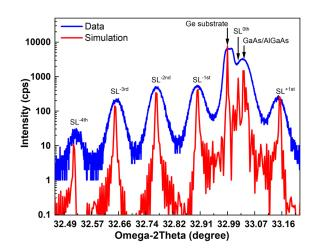
**FIG. 3.** XRD  $\omega$ -2 $\theta$  scan of the SML QD-QCD sample grown on Ge. The blue curve represents the measurement data, while the red curve is the simulation result.
